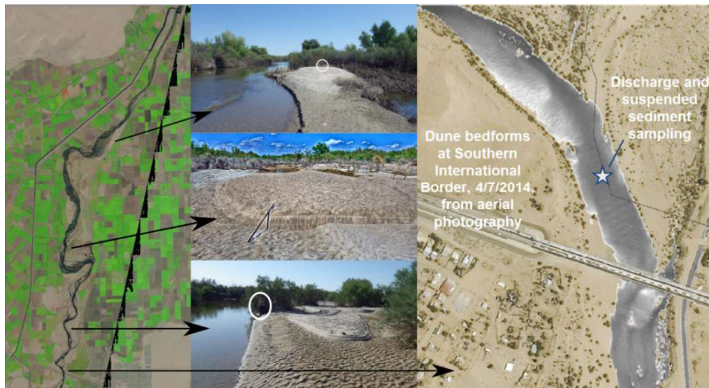
Figure 6 Landsat image from 3/31/2014 during the peak of the pulse flow and examples of sediment deposition and bed forms because of the pulse flow. Backpack (circled), 2 m rod in foreground, and person (circled) for scale. Width of channel is approximately 300 m in the Worldview panchromatic image at right.
